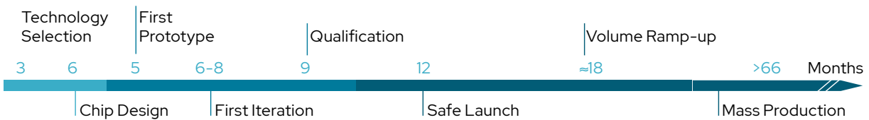
Fig. 4.5: Illustrative lifecycle for automotive: Analog/mixed-signal products are much more specialized for their applications and are used for many years
